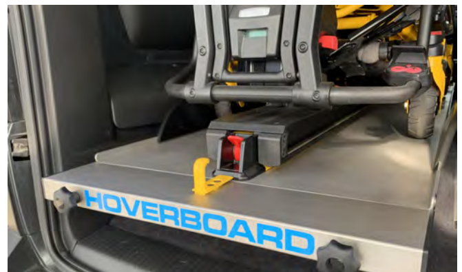
EMERGENCY OPERATION Plate extension is mounted
