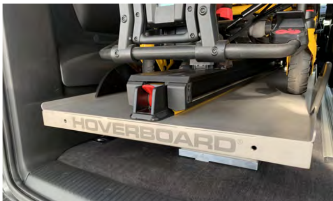
NORMAL OPERATION Plate extension stowed in the vehicle
